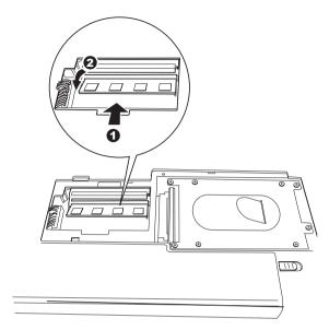
Installing the memory module
